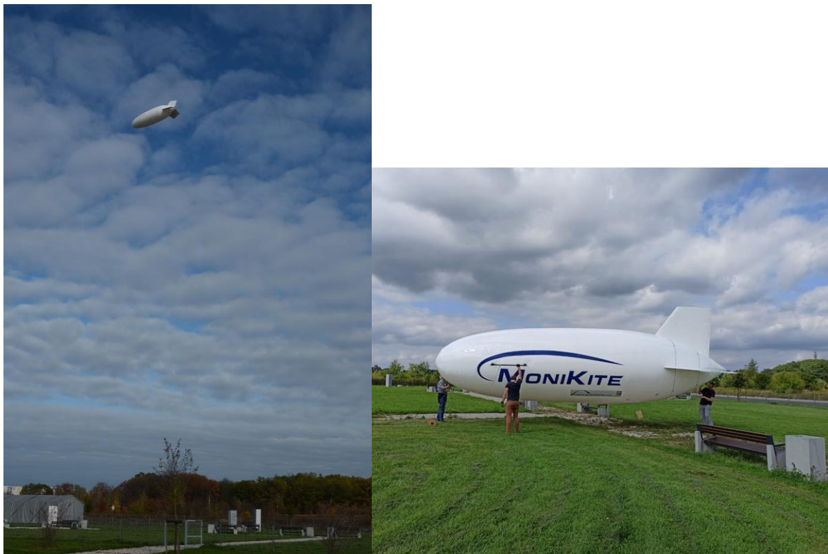
MoniKite-105 aerostat a) ca. 50 m above the ground at operation altitude, b) on the ground
